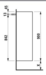
X =The exact hight must be set during installation.
